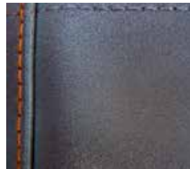
The integrity of the reflective tape is secured for 50 cycles of washing and drying at 60°C
