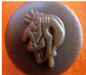
The buttons are part of the oven test in the EN ISO 11612 standard where all accessories are placed in an oven at 180°C during 10 minutes (testing of F symbol), after which the integrity of the accessories need to be in operating order.
