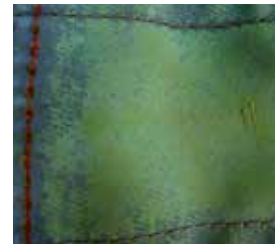
Reflective tape that lost all of its glass pearls after only 3 cycles of washing "in accordance with the neck label"; turning it green in colour.
